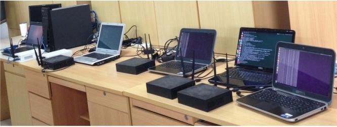
Fig. 2. Broadcast testbench consisting of USRP-based CR nodes and smart jammers.
