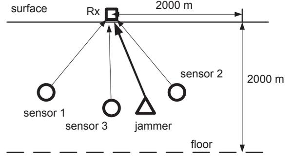
Fig. 1. Topology of an underwater sensor network against a jammer.
