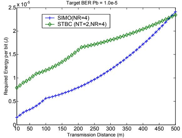
Fig. 4 Total energy expenditure of SIMO and STBC in SENMA without throughput constraints
