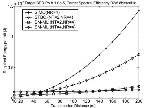
Fig. 5 Total energy expenditure of SIMO, STBC and SM-ML in SENMA with throughput constraints
