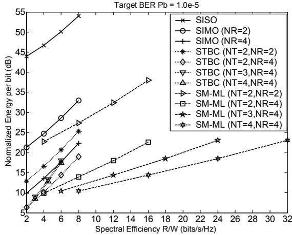
Fig. 2 Realistic systems with Rayleigh fading
