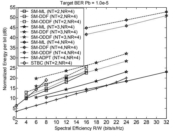
Fig. 3 Comparison of spatial multiplexing schemes in Rayleigh fading
