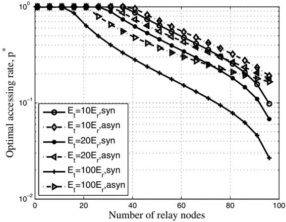
Fig. 1. The optimal channel access probabilities for energy-efficient broadcast, for both the synchronous and asynchronous relays, with  $C = 256$  and  $N = 100$ , as given by Lemma 3.2 and Lemma 3.3.
